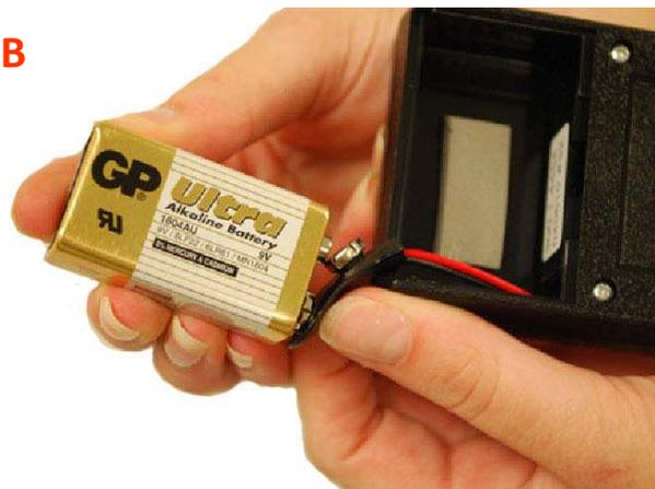
Your ReBuilder<sup>®</sup> is powered by a pre-installed 9 volt battery. The battery is located in the back of the ReBuilder<sup>®</sup> unit. To open, press down with thumb on the ridged section and slide from the bottom of the unit. (figure A)
