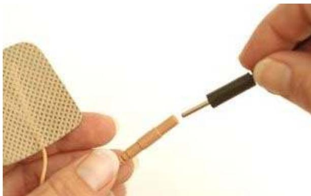
To replace the adhesive pads, grip the plastic end of the black lead wire and the plastic end of the adhesive pad and pull apart with a slight twisting motion.
